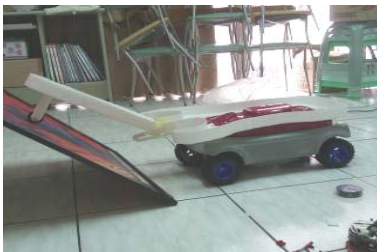
Figure 11. The front part lifts when encountering obstacles
