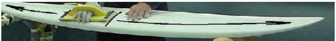
(w) When shaping the deck it is necessary to make long continuous movements with a hand that holds the shaping tool and check possible bumps with another hand.
