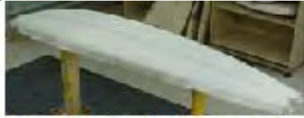
(a) Board is placed on the rack, and its bottom part is covered with a piece of cloth. The cloth is cut with about 2.5cm of excess on each end
