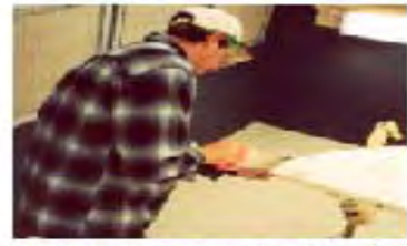
(c) Cutting and trimming the tail and nose.
