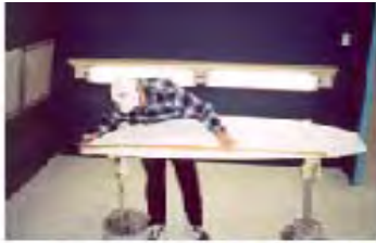
(a) Drawing the shape of the surfboard on one side of the blank.
