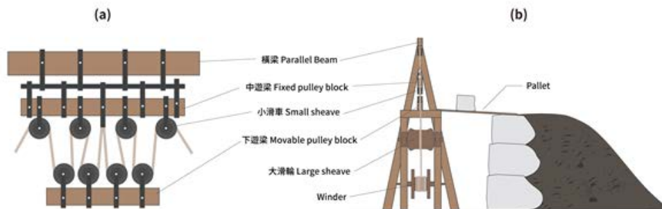
Figure 4. Pulley System of Geojunggi (a) and the construction of fortress walls utilizing Geojunggi (b). (Created by the author)
