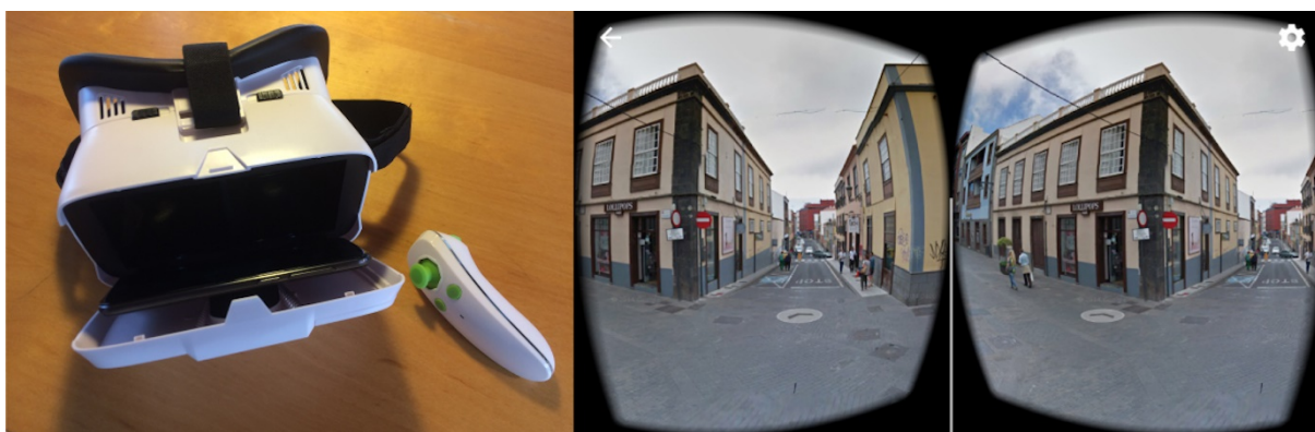
Figure 1. Left: Woxter Neo VR glasses. Bluetooth remote control with joystick. Right: Virtual urban environment generated.
