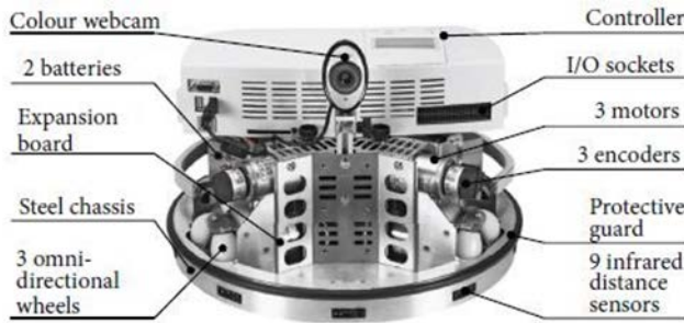
Figure 12. Mobile robot (photo from Robotino manual (Bliesener et al., 2007))
